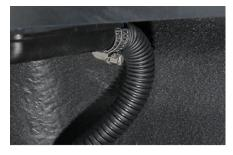
Any water entering the canister is drained to the road
