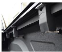
Triple clamping system, rails bolt to the clamps, and clamps bolt to the tub
