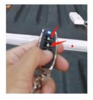
Then immediately after the fuse is re-installed (you have 5 seconds to do this) press both "open" & "close" buttons at the same time (shown in the photo with the red arrow pointing to them), do this for one or two times until you hear a "DIDI" sound. The "DIDI" sound means the code match was successful and the remote is programmed.
